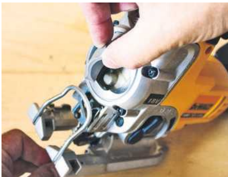
▲ This large, easily operated flush-fitting lever releases the blades
